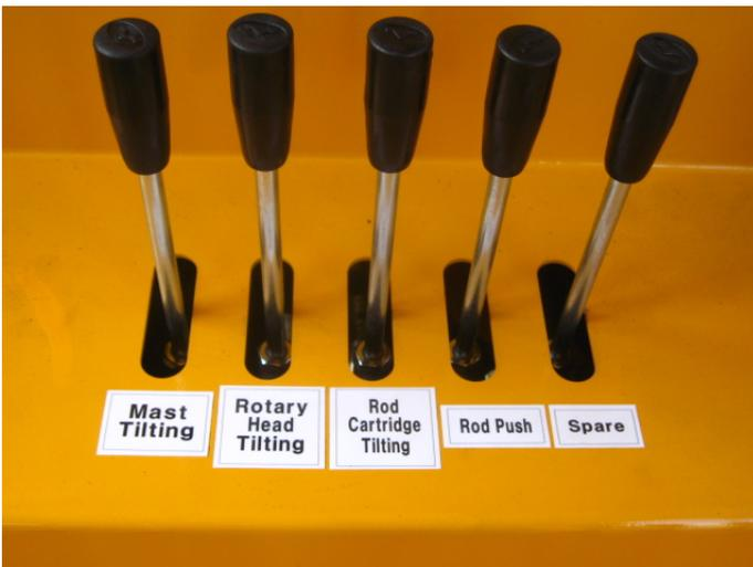
**Mast tilting :** Mast tilting for the drilling tool installation.
