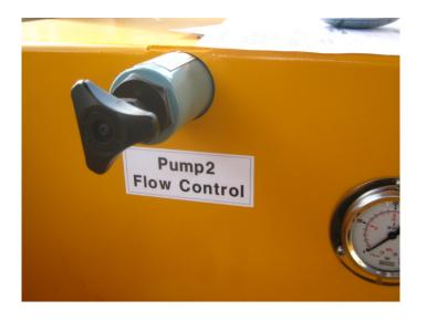
Pump 2 flow control for the rotation speed control.
