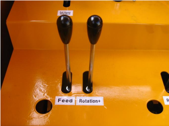
**Feed** : Fast up / down of the rotary head for rod changing.
