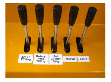
Mast tilting : Mast tilting for the drilling tool installation. Rotary head tilting : rotary head tilting for the drill rod changing. Rod cartridge tilting : The rod cartridge should be adjusted for the rod changing. Rod push : For the rod connection, Rod can be push up a little. Spare : Spare port.
